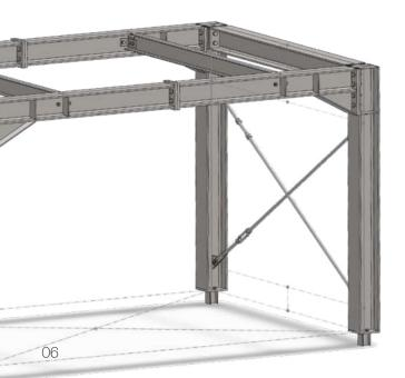
In addition to connections, steel structures typically include bracings such as cross bracings, K-bracings, and other shapes. SolidSteel parametric simplifies this tedious design task.
