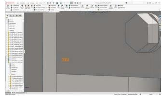
For the DXF export, SolidSteel parametric for SOLIDWORKS provides automatic, individual labeling of the parts. Thus, for example, the position number can be labeled fully automatically on all sheet metal parts.
