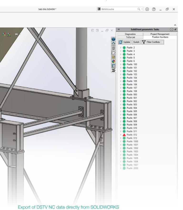
With the DSTV Assistant for SOLIDWORKS, you can export NC data from steel components (profiles and sheets) in DSTV format directly from SOLIDWORKS and pass them on to machine production.
