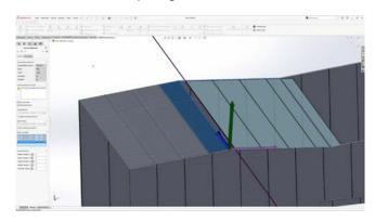
In this process, all the properties such as profile types and offsets are adopted, and transitions between the two roof surfaces are created automatically.
