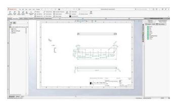
Shop drawings of assemblies and individual parts can be created as easily as parts lists with just a few clicks. In the case of individual part drawings, all dimensions required for production are automatically inserted.
